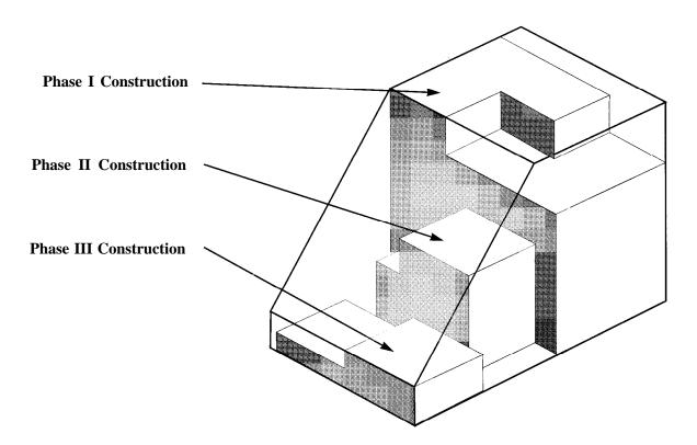
Figure 2-6: Phased Development Within A Single Solar Envelope
