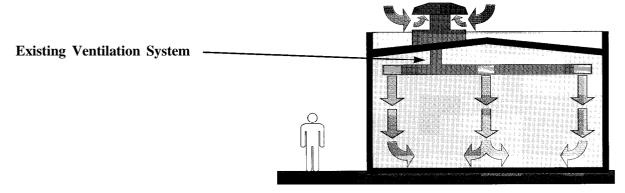
Figure 1-15: Night Mechanical Ventilation (NMV)
