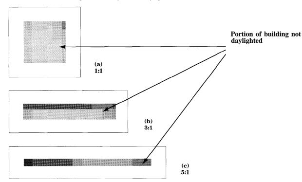
Figure 2-11: Changes in Building Shape (Aspect Ratio)
