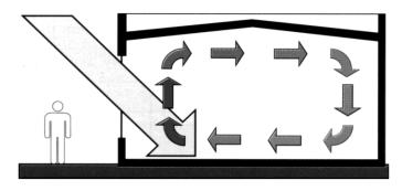
Figure 1-4: Direct Gain (DG) Schematic
