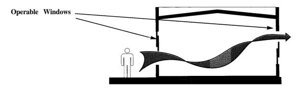
Figure 1-14: Natural Ventilation (NVN) Schematic
