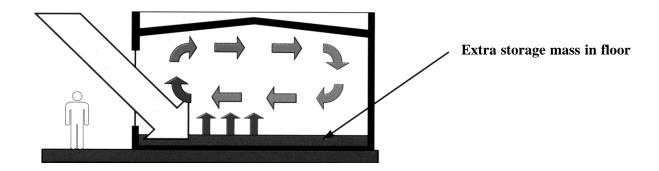
Figure 1-6: Direct Gain plus Storage (D+S) Schematic
