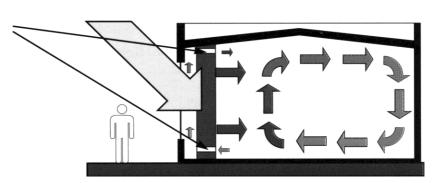
Figure 1-8: Indirect Gain (IND) Schematic
