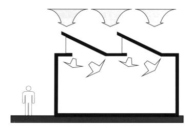
Figure 1-21: Sawtooth Aperture (SAW) Schematic
