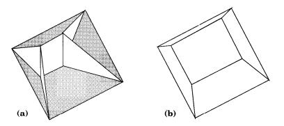
**Figure 2-5: The Final Solar Envelope**(a) final boundaries, (b) solar envelope within boundaries
