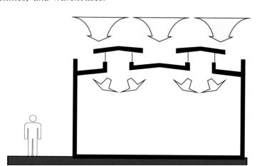
Figure 1-23: Monitor Aperture (MON) Schematic
