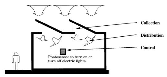
Figure 1-3: Components of a Daylighting System
