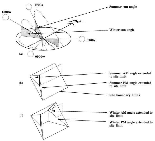
Figure 2-4: Establishing Solar Envelope Boundaries
