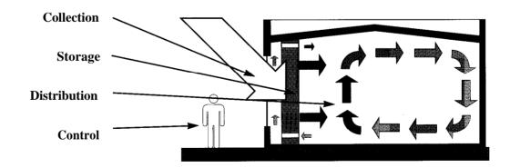
Figure 1-2: Components of a Passive Solar Thermal System
