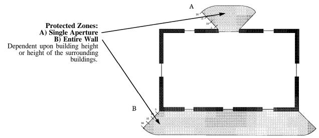
Figure 2-9: Site Planning For Daylighting
