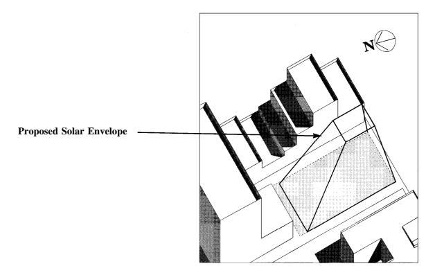
Figure 2-3: Solar Envelope For Constrained Site
